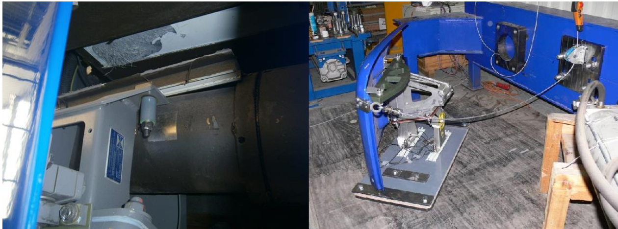
Figure 4.19 Bonding validation test of equipment fixing on rolling stock after detachment problems
