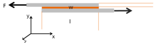
Figure 4.21 Sketch of a lap shear joint
