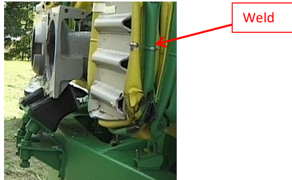
Figure 4.3 Crushed crashworthy steel devices without welds rupture
