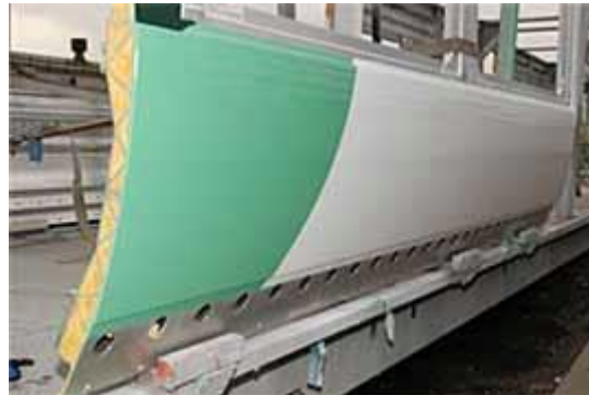
Figure 4.7 FSW welded Side walls of aluminium rolling stock by Bombardier
