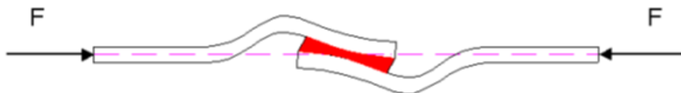
Figure 4.20 Unstable design of an adhesive joint due to local buckling in the overlap
