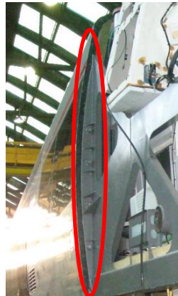
Figure 4.10 Steel Driver cab bolted on the current aluminium carbody
