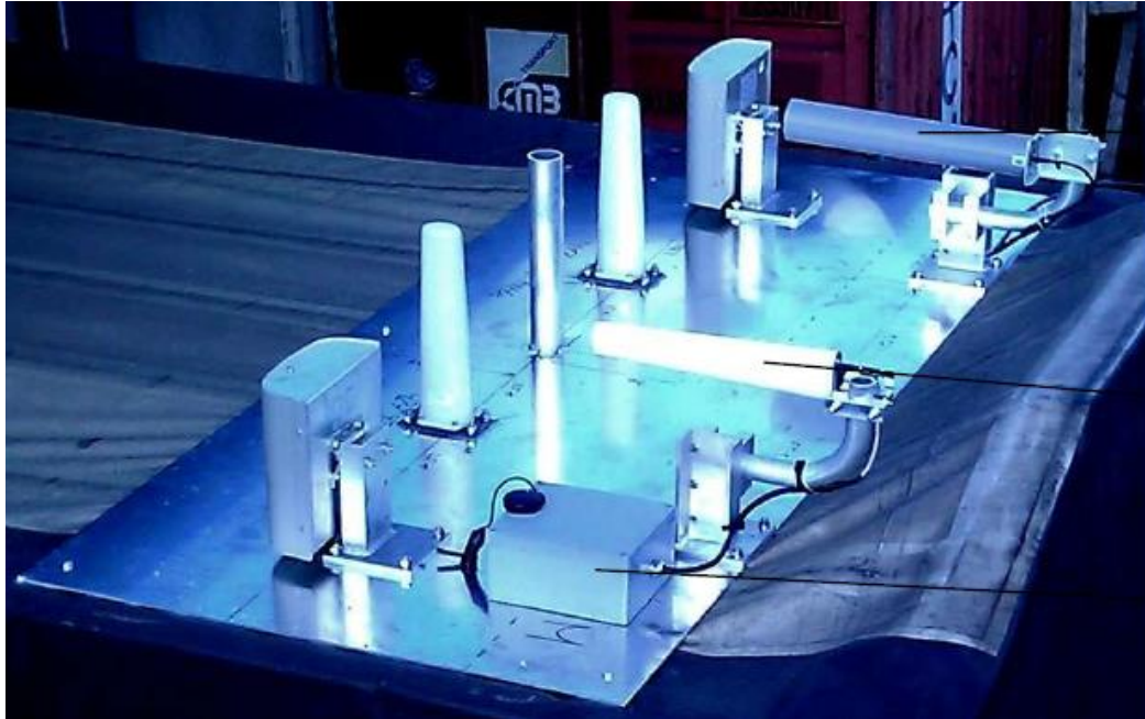
Figure 4: Set of antennas used in the first radio test
